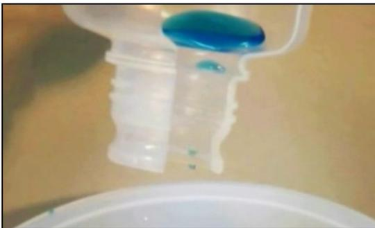
Accumulated plastic at neck often interferes with smooth pouring and complete drainage in EBM bottles
